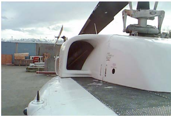
Figure 7-5 Engine Air Inlet
